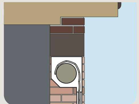
When the reveal fix option is chosen it may also be necessary to strengthen the lower edge of a 90° fascia when fitted partially or fully into a garage door opening, in order to prevent it from marking the door's curtain during operation.
